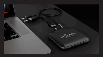
I. Connect the transmitter unit to your device via the HDMI port and to a power source using the USB Cable
